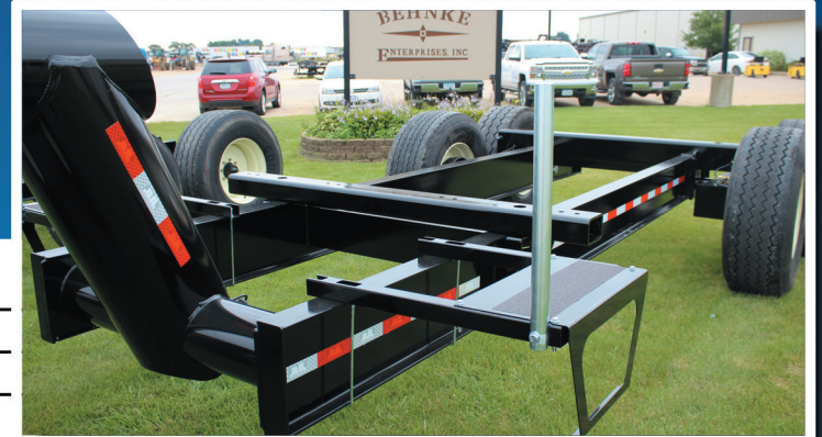
Repositionable step, each side.
